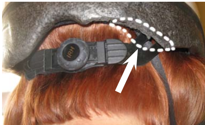
The back of Jean Riggs's helmet after a fall, showing a large chunk missing.
